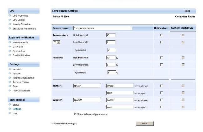
The environment sensor measures temperature, humidity and gives the status of the 2 contacts (used for door, alarms or generator unit).
